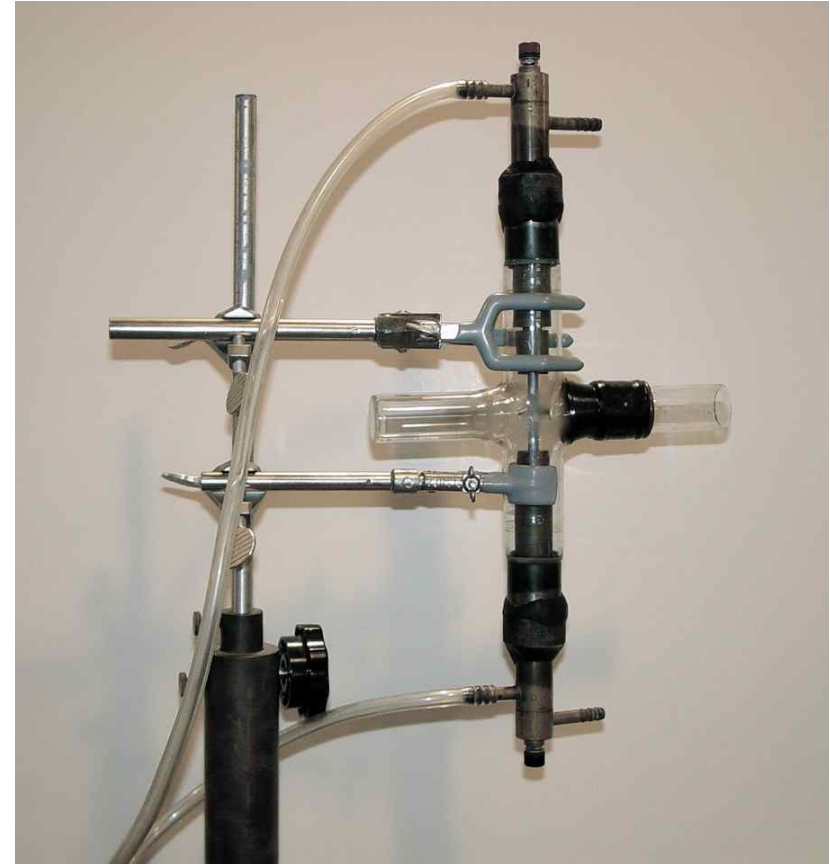
Sliding spark source used to excite doubly-ionized through seven-times ionized spectra.
