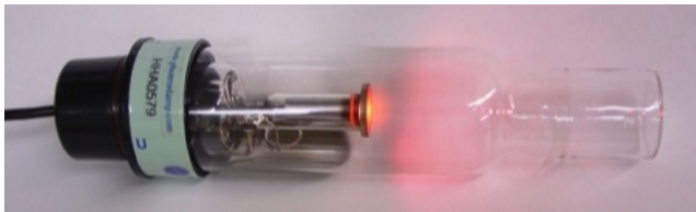
Commercial (10-20 mA) hollow cathode lamp
